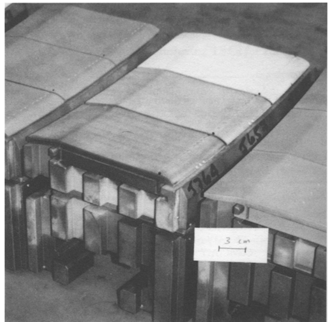
Fig. 4 Photograph of thermal barrier coated MS7001FA shrouds in outer shroud hangar prior to installation into machine
